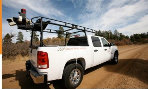
GeoNav's vehicle mounted 3D mobile mapping IP-S2 system maps rural America.
